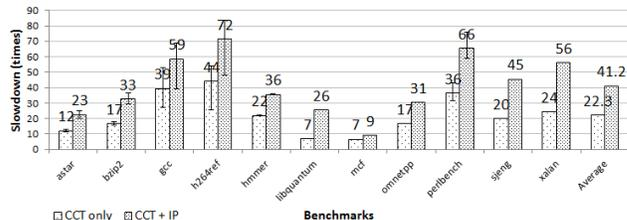
Figure 6: DeadSpy overhead for SPEC CPU2006-INT.
